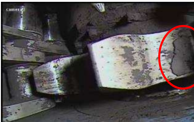
Coal consolidation impacted by flow discontinuity
