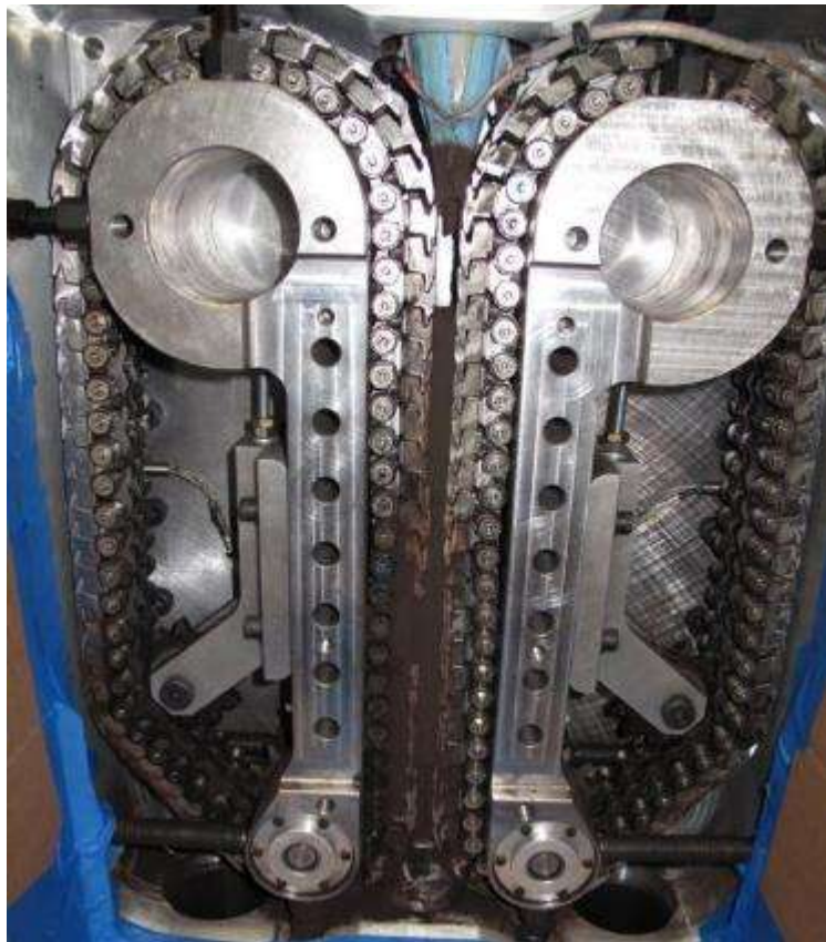
Initial Tile-sidewall Leakage Addressed by Side Seals and Vacuum Clearing Ports
